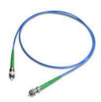
These polarization-maintaining fiber optic patch cables are terminated on both ends with high-quality, narrow key, ceramic FC/PC connectors, featuring high-quality polish with a typical return loss of 50 dB. Each cable is individually tested to ensure the specified extinction ratio and insertion loss at fiber-to-fiber junctions. Each patch cable includes two protective caps that shield the ferrule ends from dust and other hazards. Each cable comes with a mating connector adaptor for ease of use.
